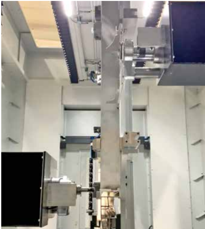
Milling spindle left and milling spindle right (under extraction bell) simultaneously in use on two sides
