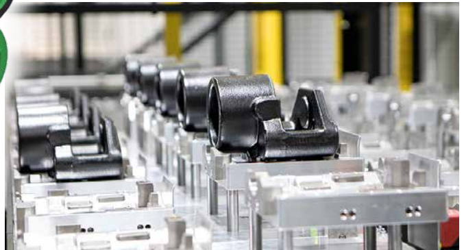
30 parts self-sufficiency – infeed conveyor as pallet accumulation conveyor
