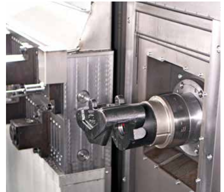
Workpiece on OP20 mandrel for rear machining
